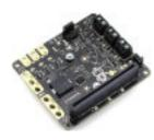
The Kitronik environmental control board provides a variety of sensor inputs and connection points for the BBC micro:bit and provides the ability to control outputs for devices such as a water pump, fan, servo or heater pad. This makes it ideal for feedback control systems.
